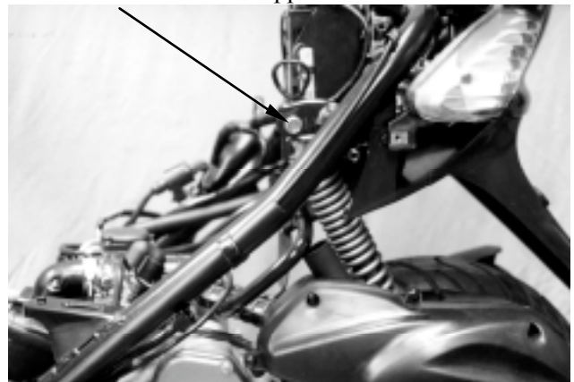
Rear Shock Absorber Upper Mount Bolt
