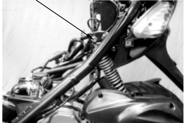
Rear Shock Absorber Upper Mount Bolt
