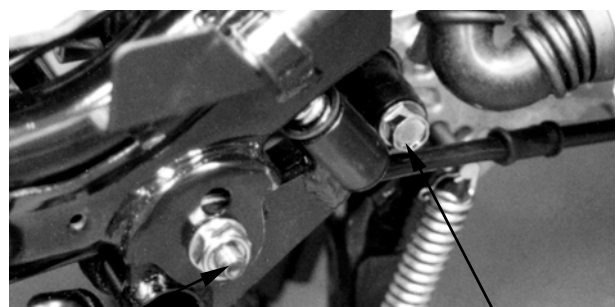
Engine Hanger Bracket Bolt
