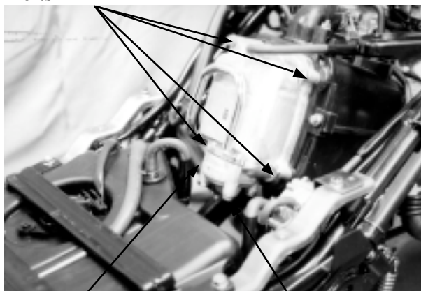
Secondary Air Inlet Tube Bolt
