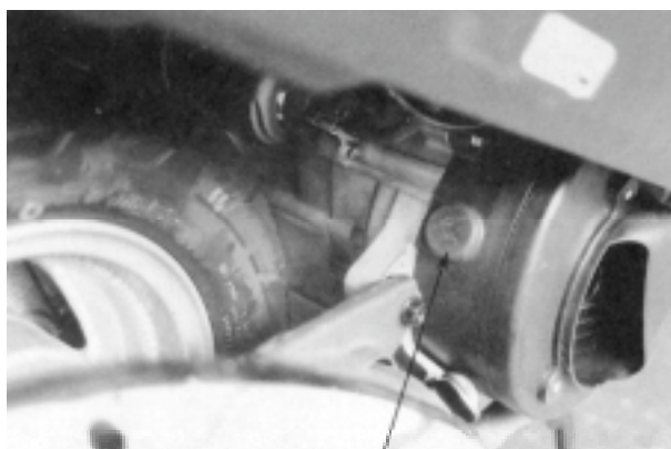
Timing Hole Cap
