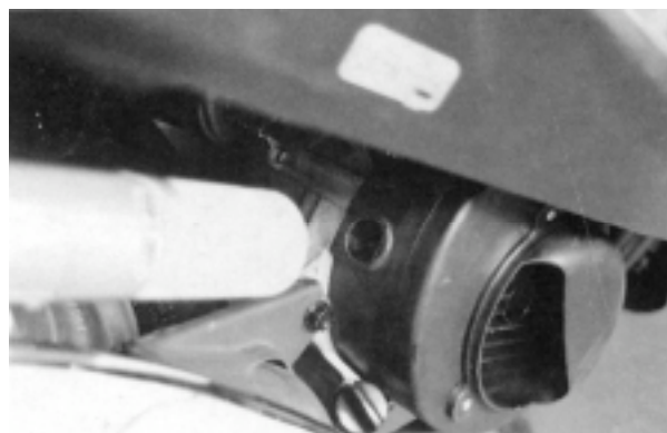
Timing Hole Cap
