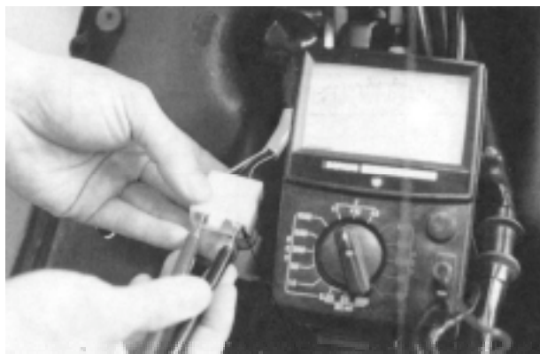
Ignition Switch Coupler
