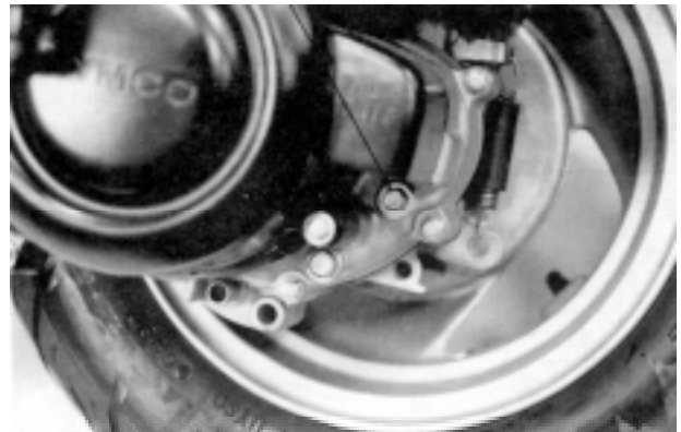
Oil Check Bolt/Sealing Washer
